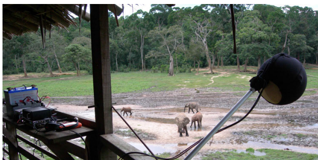
Figure 2: Testing the recording system for a 24-hour continuous 8-channel recording in the saline of Dzanga Bai, Africa, 2008. (Photo: D. Monacchi)
